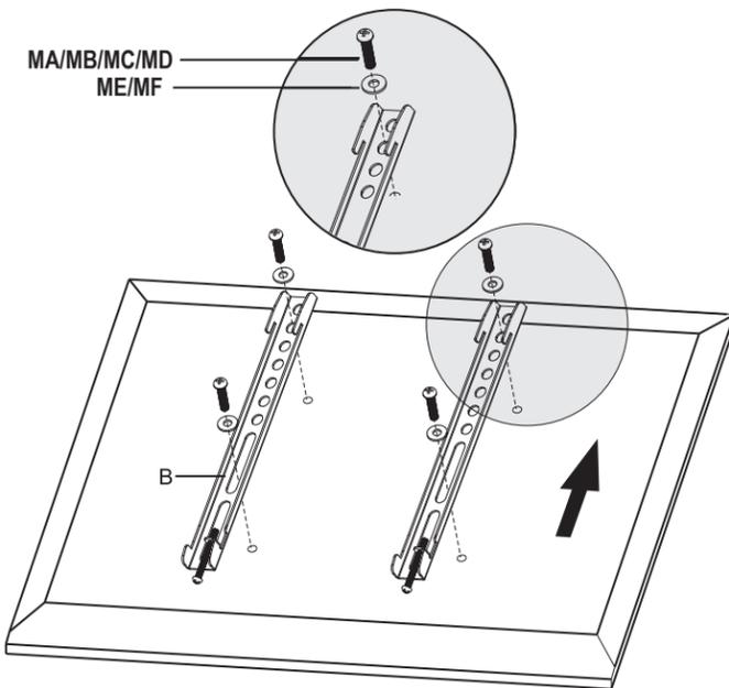
2. Install the screen onto the stand.
