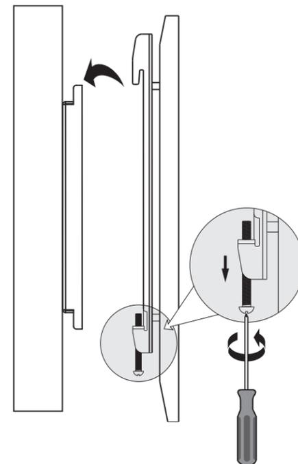
Loosen the inferior screws to mount the screen easily.
