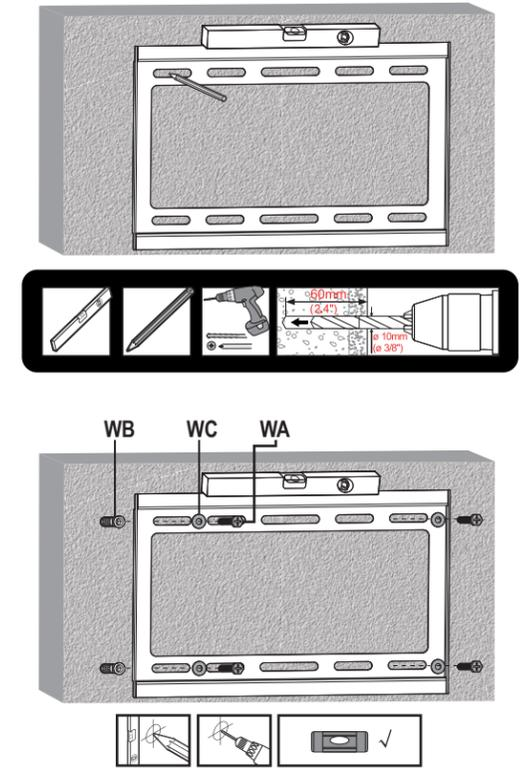
Before drill, make sure that does not exists electric wire pipes, gas or water.
